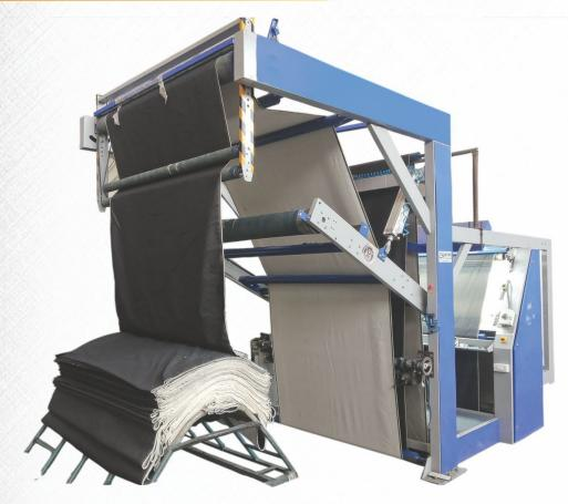
$\mathscr{G}_{t's}$  a Combi machine, where fabric can be feed in Roll or Fold form and it can deliver in Big-Batch form or Fold form. Due to its possibilities it saves lots of space and never stay idle. A mandatory machine for any inspection and make-up department.
