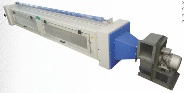
**%**-Tex Brushing & Beating Machine is a reliable tool to remove working impurities from fabric. It brushes and beats the fabric and all the dust is taken away by high pressure suction device. Modular Design of BIM-BR+BT allows to fix this unit by means of just 4 bolts on any existing machine like, Stenter, Sizing, Calendar, Inspection, etc.
