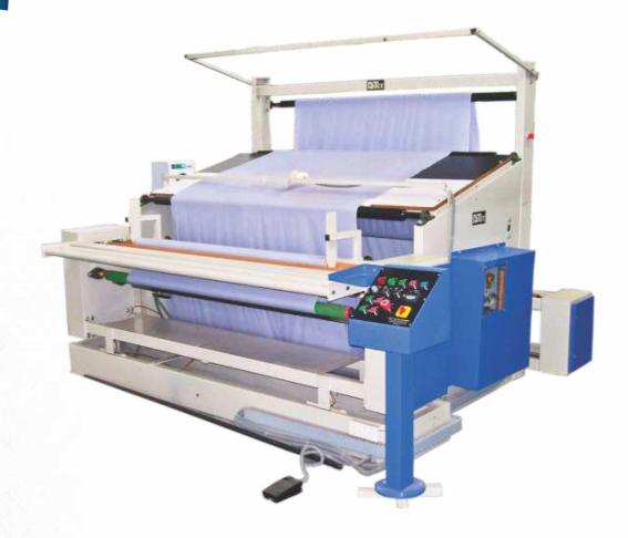
Opecially designed to mend the fabric with ease and space concern. BIM-RR is very economical machine where operator can easily sit and mend the fabric for hours without stress. Finally fabric is delivered in roll form without wrinkles and appropriate guiding. Driven Un-winder can be incorporated for rewinding or Heavy Rolls. Also horizontal table is possible with back light for mending purpose.
