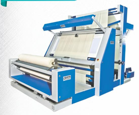
. Yumbo Rolls can be easily Inspected and rolled as per desired length in this special designed machine. All the Drives are synchronised and ensures tensionless handling of fabric.
