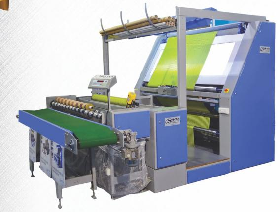
Multifunction inspection machine, with the simplicity of single person operation. BIM-RR+CD can Inspect, Measure, Auto-Cut, Auto-Eject and Conveys the presentable fabric rolls to packing, resultant benefit is auto transportation, time savings, educed manpower & space needs, increased production and finally saves costs too. It ensures minimum wastage and high quality delivery of fabric, also tensionless handling for enhanced fabric care, single operator run are some of the additional benefits
